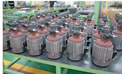
▲T-rotor pump 조립 Line
